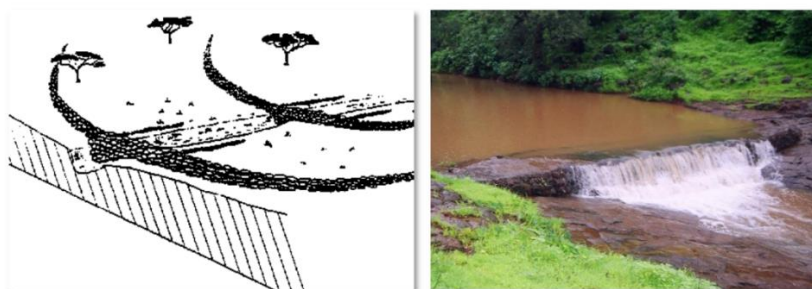
Figure 10. Concept of a cascade to permeable weirs (left) and an example of a permeable weir made of gabion baskets.
